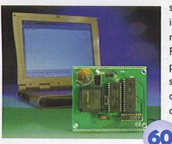
system. Its most important features in this regard are on-board Flash memory programming via the serial RS232 port, direct on-board program debugging and low cost.
